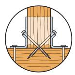
Replace double shear nails with SD #9x2½" screws
