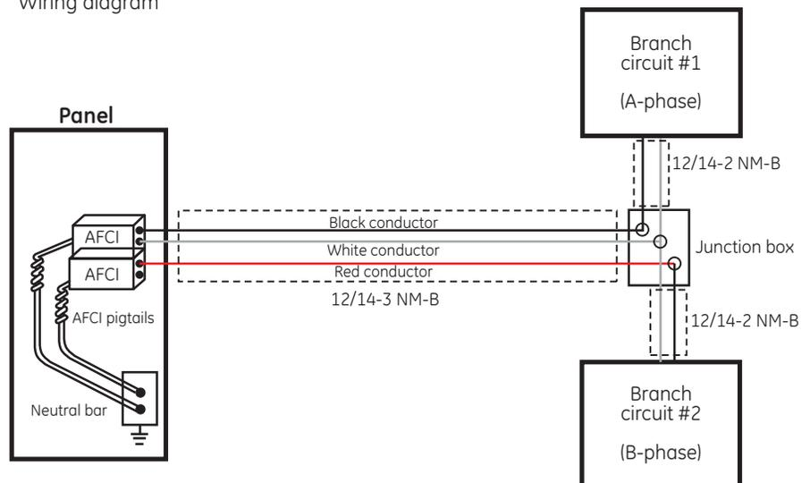
*Note: for simplicity the ground wires are not shown*
